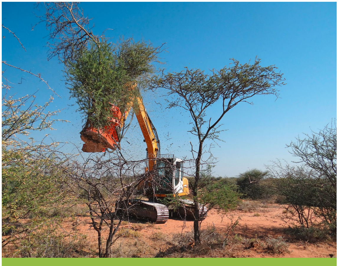
Mechanised harvesting of encroacher bush
